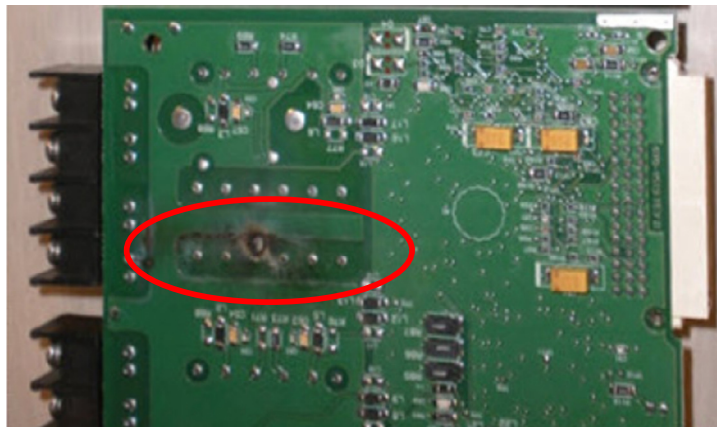
Damage from arcing caused by overvoltage from open circuited CT. Photo from White Paper "Open-Circuited CT Misoperation and Investigation" [2]
